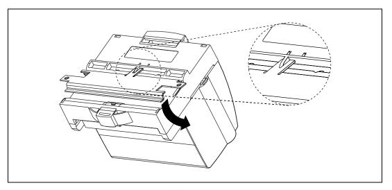
Figure 2-3. Installing the Network Panel Mount Accessory
